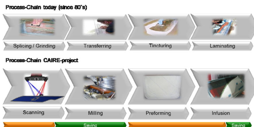
Figure 1-2: Comparison of repair process-chain.
